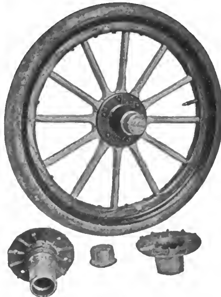
DETAILS OF THE SALISBURY WHEEL AND HUB.
